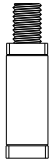
R1 (ADS7134) Fit 3/4 Square Tube Exp. 0.720 - 0.851 1/4 Square Metal Top Round Rubber 1/4 Square Metal Base
