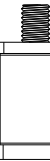
U5 (ADR7538) Fit 1-3/8 Square Tube Exp. 1.360 - 1.425 1/4 Square Metal Top Round Rubber 1/4 Square Metal Base
